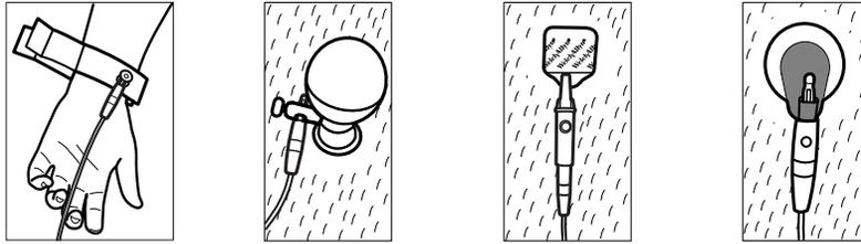
Electrode examples, left to right: arm clamp (reusable), Welsh cup (reusable), tab electrode (disposable), monitoring electrode (disposable).
